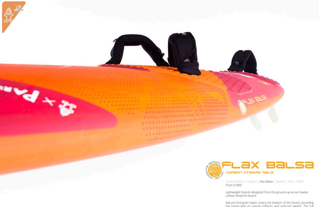
Natural end-grain balsa covers the bottom of the board, providing the board with its overall stiffness and reduced weight. The full sandwich deck uses natural uni-directional flax fibres with carbon stripes to reinforce and stiffen the most stressed sections. Wave models add a full-perimeter Carbon-Innegra rail band for extra strength
